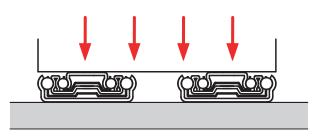
Horizontal installation of the telescopic slides is partly possible as well. The load values are approx. 50-60% less than for vertically mounted guides.
