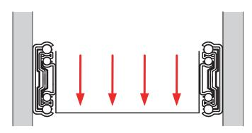
Vertically mounted telescopic slides are distinguished by super-imposed ball tracks. This special design makes them extraordinarily torsion resistant and increases the service life and the carrying capacity of the guides significantly.
