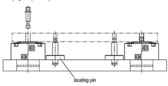
Simultaneous clamping and positioning of a workpiece
