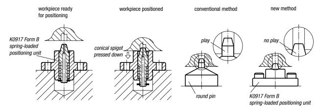
The conical spigot is pushed down when the workpiece is mounted on the positioning unit.
