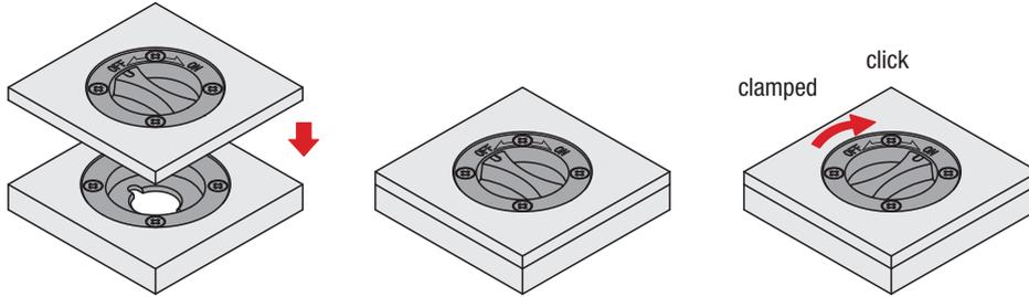
Ensure that the twist grip is in the „OFF“ position. Insert the quarter-turn clamp lock into the clamping plate and turn the grip to the 'ON' position. When fully clamped, an audible click will be heard.
