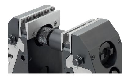
Clamped blank. Sure set-up through positive clamping pins.
