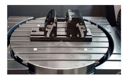
Positioning directly on the KIPP zero-point clamping system with integrated clamping pins in the 5-axis vice compact baseplate.
