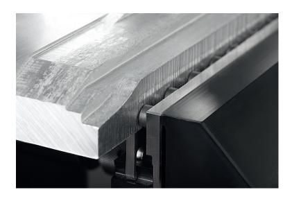
Blank after clamping. Clamping pin imprint is visible on the edge of the workpiece.
