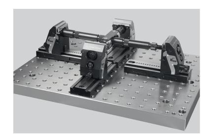
5-axis clamping system compact positioned directly on the machine table.
