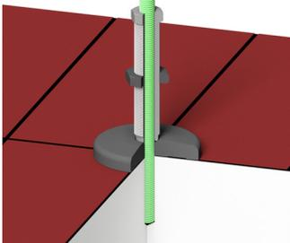
4. The levelling foot and the machine are now fully secured (no visible holes in the floor).
