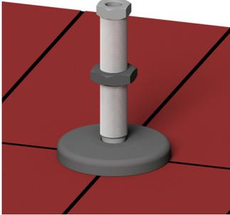
2. Once the levelling foot and the machine are positioned correctly, drill a hole in the floor through the hollow screw.
