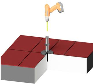
3. Insert a stud or pin through the hollow screw into the floor and secure it (e.g. with glue).
