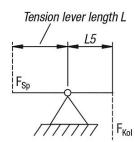
Effective clamping force  $F_{\text{Sp}}$  is dependent on piston force  $F_{\text{Kol}}$  and tension lever length L
