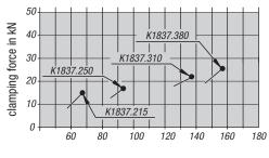
Tightening torque (Nm)
