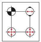
Centring pins = Form A fixes in x and y axis (reference point)
