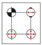
Centring pins = Form A fixes in x and y axis (reference point)
