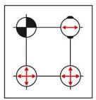
centring clamping bolt = Form A
