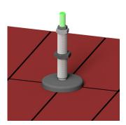
4. The levelling foot and the machine are now fully secured (no visible holes in the floor).
