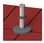
1. Place the levelling foot in the position intended for the machine.
