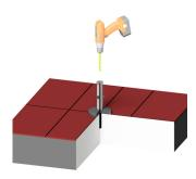
2 Once the levelling foot and the machine are positioned correctly, drill a hole in the floor through the hollow screw.
