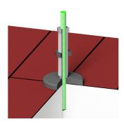
3. Insert a stud or pin through the hollow screw into the floor and secure it (e.g. with glue).
