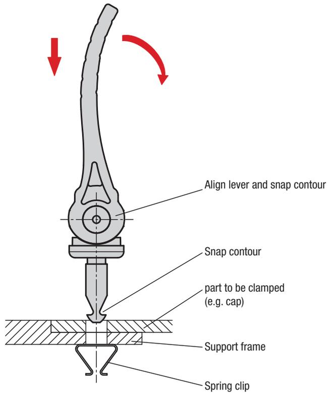
Loosen by swivelling and turning
