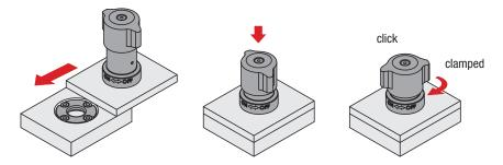
Check that the twist knob is in the "OFF" position and that the pin is retracted. Place the ball lock pin over the receiving bush or insert it. Press the twist knob down and turn it to the "ON" position. When fully clamped, an audible click will be heard.
