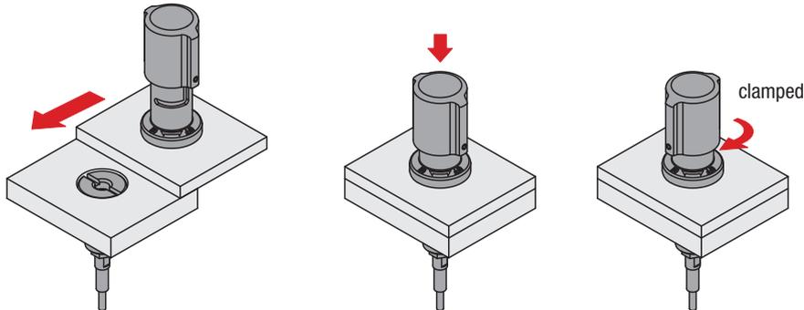
Check that the twist knob is in the „OFF“ position and that the pin is retracted. Place the ball lock pin over the receiving bush or insert it. Press the twist knob down and turn it to the „ON“ position. When fully clamped, an audible click will be heard.
