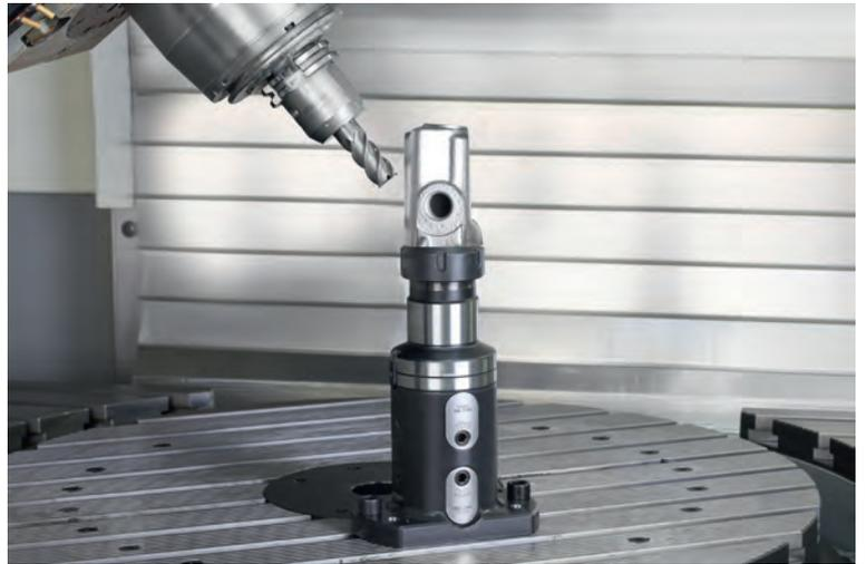
Gearbox housing mounted on 3 basic modules, 3 add-on modules and 3 reducer adaptors. The cast housing is secured to the reducer adaptors by means of socket-head screws.
