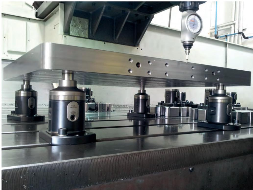
4 basic modules H=100 positioned directly on the machine table. The 4 reducers H=50 on top facilitate optimum access to workpieces.
