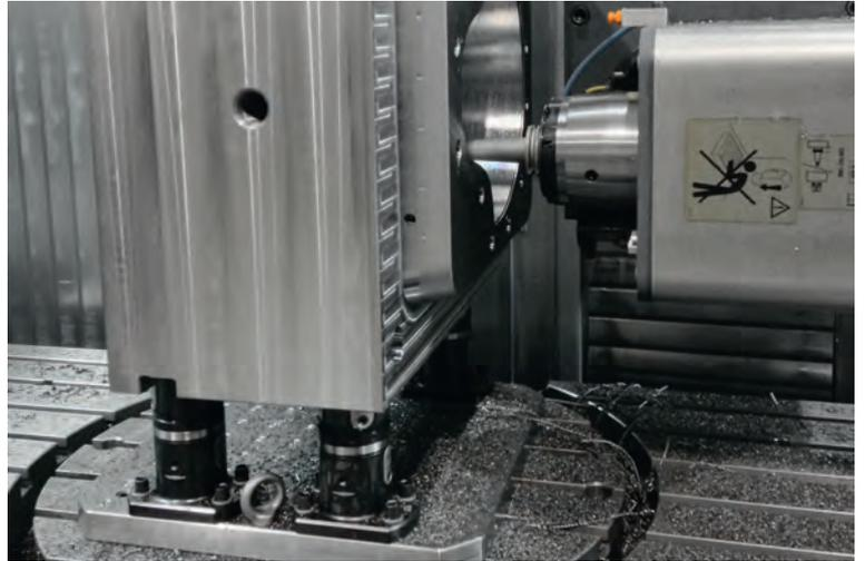
2 basic modules with a centring clamp adapted directly to a zero-point clamping system.
