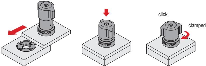
Check that the twist knob is in the „OFF“ position and that the pin is retracted. Place the ball lock pin over the receiving bush or insert it. Press the twist knob down and turn it to the „ON“ position. When fully clamped, an audible click will be heard.
