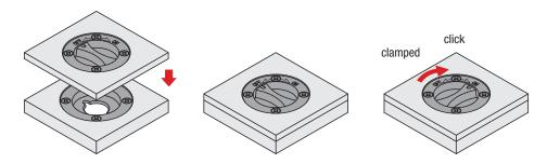
Ensure that the twist grip is in the "OFF" position. Insert the quarter-turn clamp lock into the clamping plate and turn the grip to the 'ON' position. When fully clamped, an audible click will be heard.
