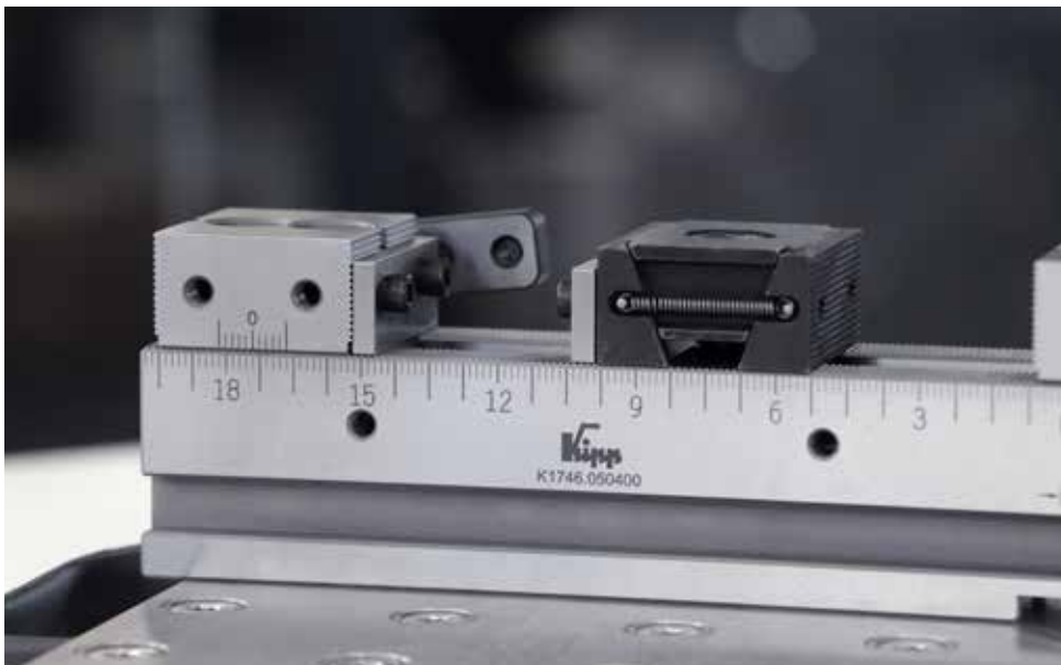
Multi-clamping system with support bars and lateral workpiece stop for the workpiece.
