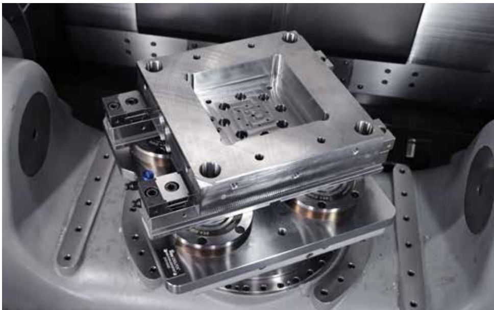
Workpiece clamping with fixed jaw (right) and wedge clamps with fixed jaw (left).
