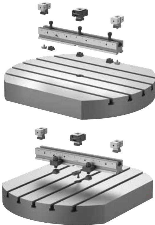
Mounting of the multi-clamping system along and across a T-slot machine table is possible. Alignment with slot keys. Secured using screws or clamping claws.
