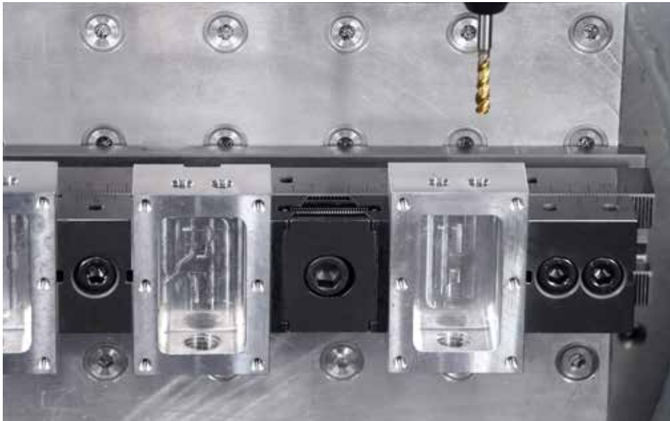
The multi-clamping system with wedge clamps double-sided and various fixed jaws combined.
